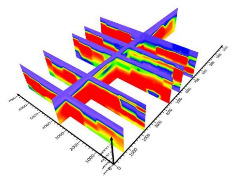
Create multiple image slices to show how data changes along survey lines or at specific orientations.
