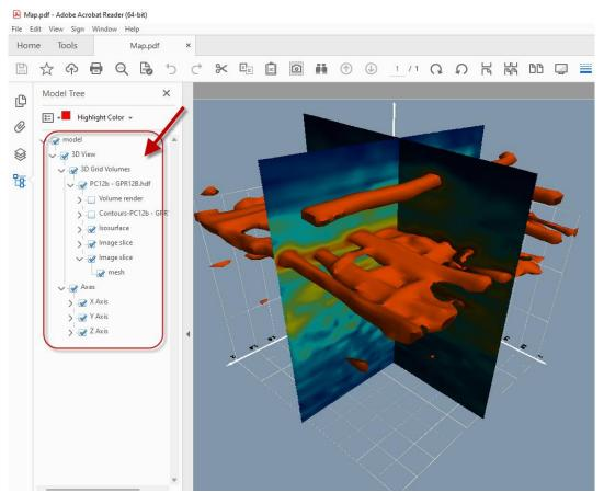
Open the 3D PDF exported from Surfer's 3D View and all the components of your model are logically grouped together in the Model Tree so you can easily turn them on and off.
