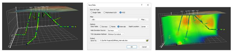
Import drillhole data and visualize it in 3D. Save the data directly from the **Drillhole Manager** and grid it to create a 3D grid. Add the 3D grid back to the model to view the interpolated data.
